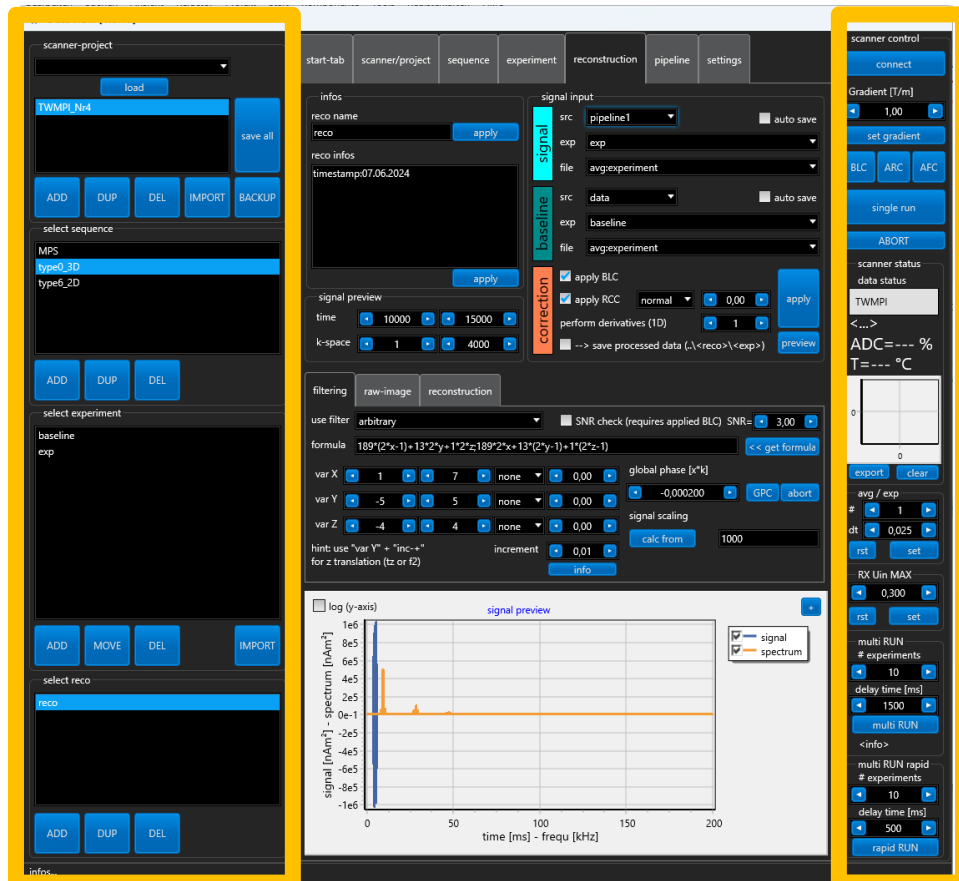
Figure 1-1: Screenshot of the main window of the software. Left: overview of the projects and their sub-categories. Center: For each category, a separate page is provided with additional parameters. Right: scanner control panel with access to scanner parameters and experiment control.
