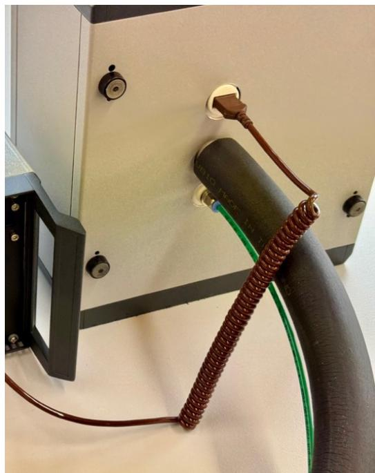
Please be advised that the 6 mm tube connecting the "Air Out" port of the VT control should not exceed a length of 60 cm. If this connection is kept short, heat losses are reduced, and a lower temperature can be achieved. It is also strongly recommended that this connection is thermally insulated, in particular when working at low temperatures.
