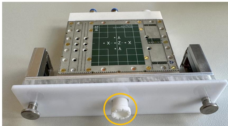
Finally, position the probe in the magnet.
