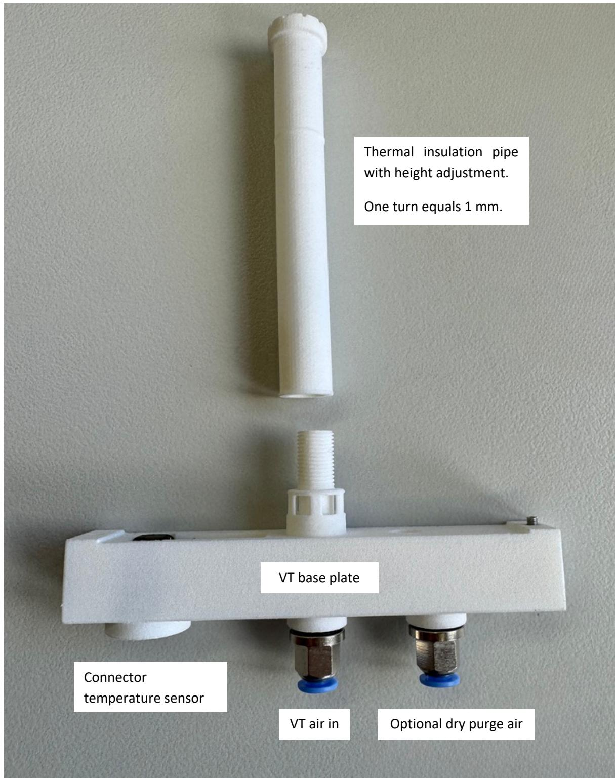
The VT base plate is equipped with a connector for the integrated thermocouple temperature sensor and two inlets for air connection.
