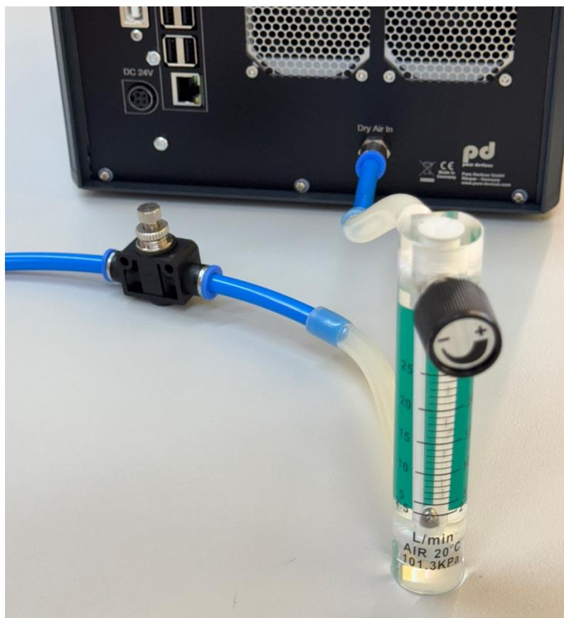
When the VT control unit is turned on and no temperature sensor is connected to port 2, then a value related to the air pressure at a certain flow rate is shown on the display. This value can be used to check whether the air pressure and therefore the flow rate is changing.
