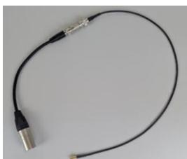
**2xXLR-to-SMB cable:** connects the Drive output (Tx2) with the Amp-N2k-compact input & connects the COMPASS lab unit output with the Drive console input (Rx).
