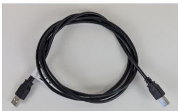
**2xUSB cable:** connects the COMPASS unit & the Drive console with the PC.
